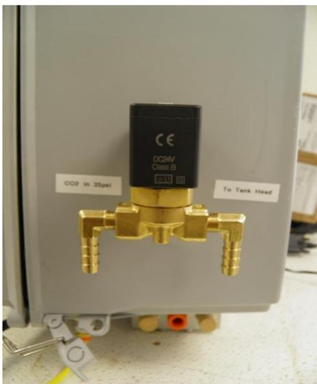
How LpC works, is when connected to a CO<sub>2</sub> source and the head space of the dispensing tank and the system is activated by pressing the “Liquid psi Control” button. The computer initially records the static liquid pressure at the manifold and displays that pressure as the set point above
